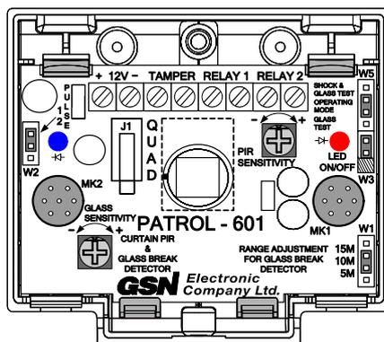
**TERMINALS "RELAY 1"** – relay output (N.C.) of the PIR detector.
